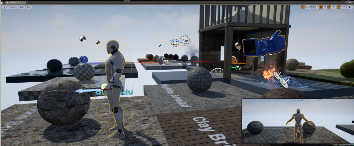
Fig. 1: The Engine2Learn UE4 plugin in action. The camera actor (blue) can be setup to send pixel observations with each step back to the ML-client, which in turn controls the agent's movements.
